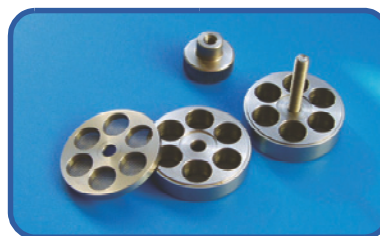
The holder has 12 sample wells
