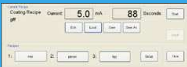
Sputtering parameters (time and current) can be pre-set and stored
