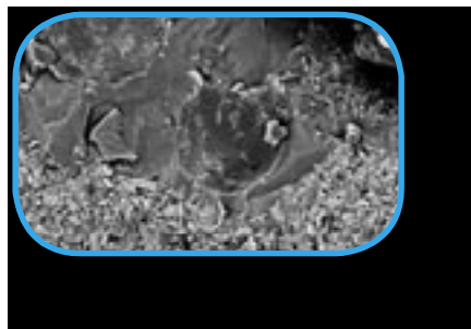
and oil. Dark grey bubbles are dried oil droplets in brine-filled cracks
